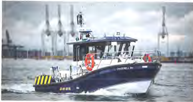
The Chasewell 9m pilot cutter was conceived for minimised environmental impact at low-speed operation
